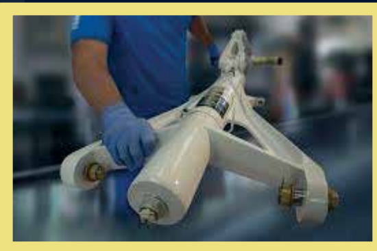
Beech craft B300 Main & Nose L/G Drag brace OVERHAUL
